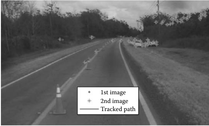
FIGURE 7.2 Point correspondences tracked in two consecutive images.
